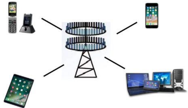
Fig. 1. Massive MIMO uses enormous antenna arrays at base stations
