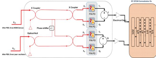
Fig. 3. The CO-OFDM receiver
