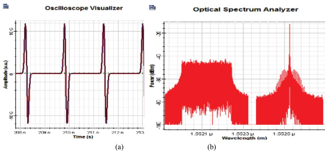
Fig. 10. The time waveform of IR-UWB based on OOK (a) and the optical spectrum of the DP CO-OFDM with DP IR-UWB (b)
