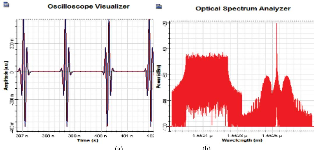
Fig. 9. The time waveform of IR-UWB based on BPM (a) and the optical spectrum of the DP CO-OFDM with SP IR-UWB (b)
