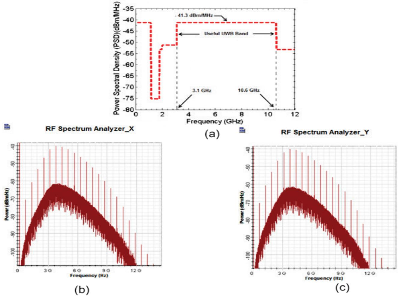
Fig. 14. Reference FCC masks UWB indoor [17] and power spectral densities of received DP IR-UWB signals
