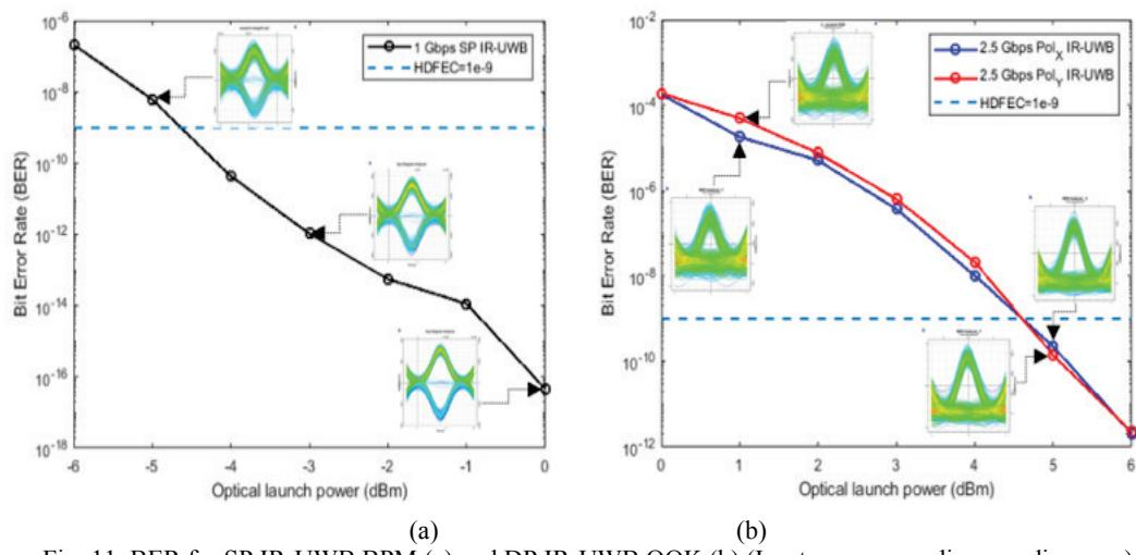
Fig. 11. BER for SP IR-UWB BPM (a) and DP IR-UWB OOK (b) (Insets: corresponding eye diagrams)
