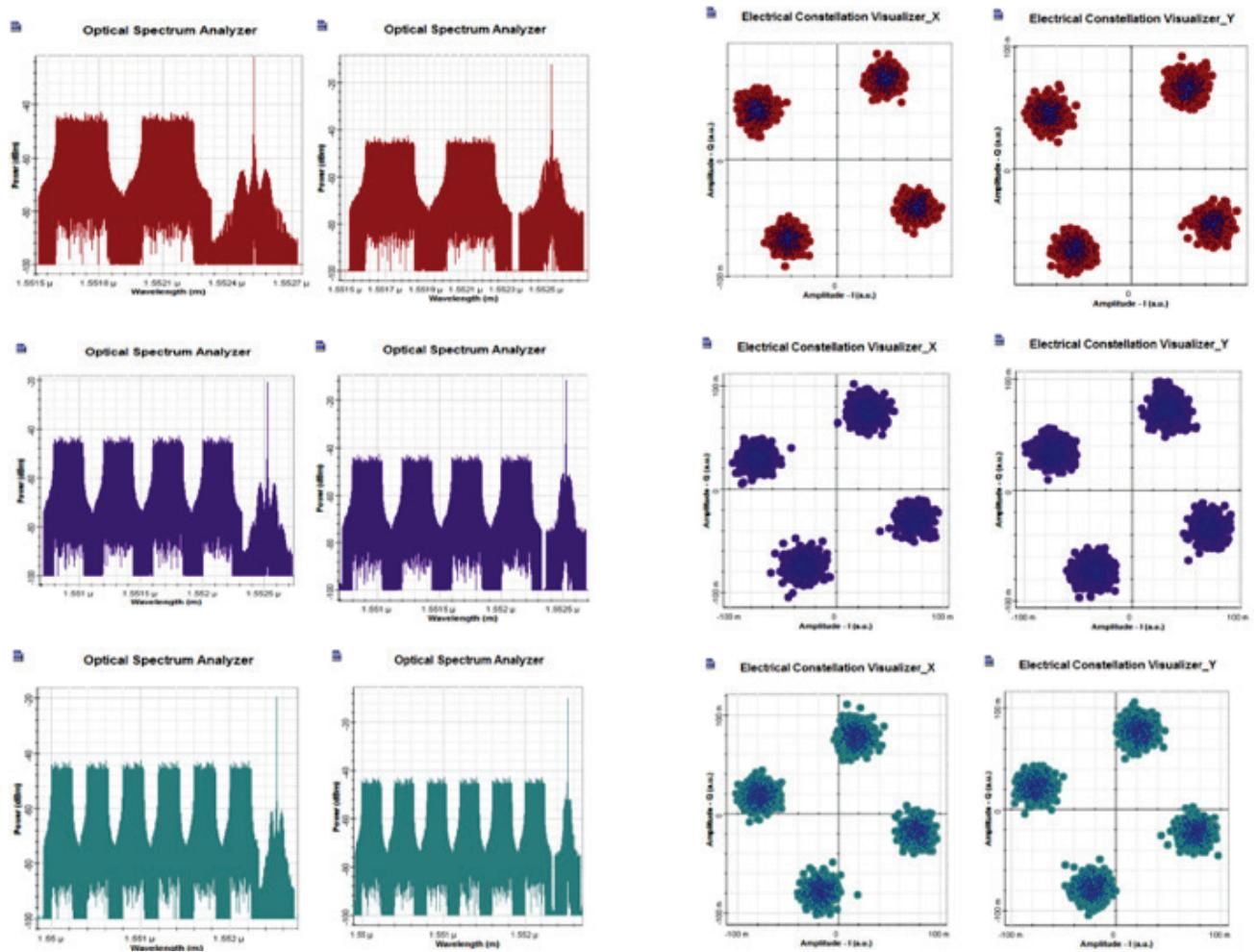
Fig. 13. Optical spectra of two, four, and six transmitted DP CO-OFDM channels integrated with IR-UWB and constellation diagrams of one DP channel
