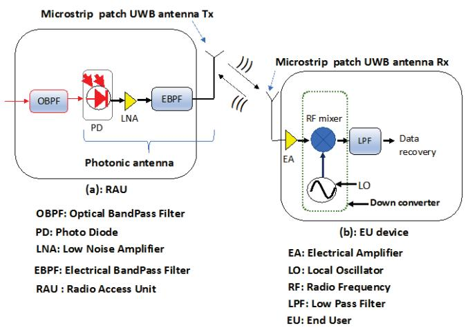
Fig. 5. The SP IR-UWB receiver with the end user device (inset in the block (f) and (g) at Fig. 1)
