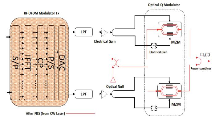
Fig. 2. The CO-OFDM transmitter
