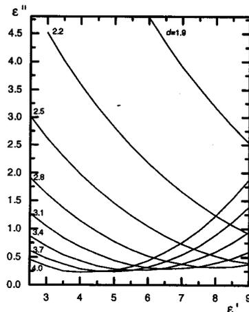
Fig. 1. Dependence  $\epsilon''(\epsilon')$  on varying sample thickness (in mm) for  $S=8$ .
