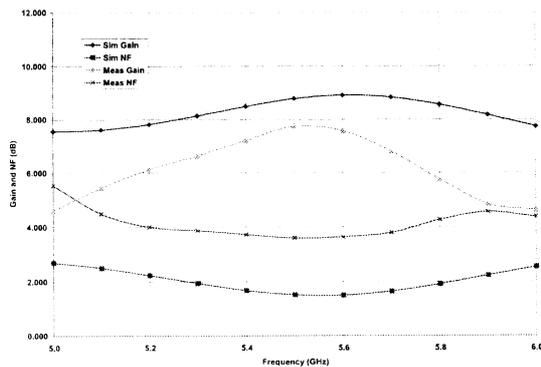
Fig. 14. Measure and Simulated gain and noise figure.
