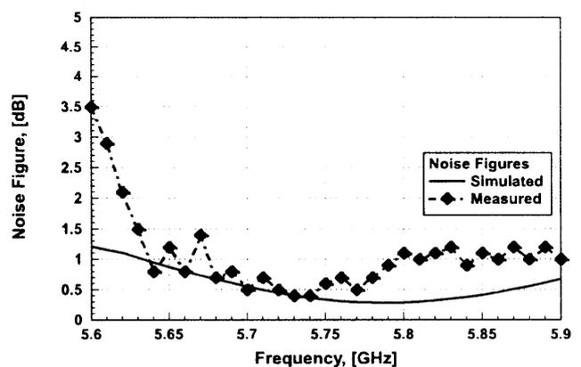
Fig. 6. Measured and simulated noise figure.
