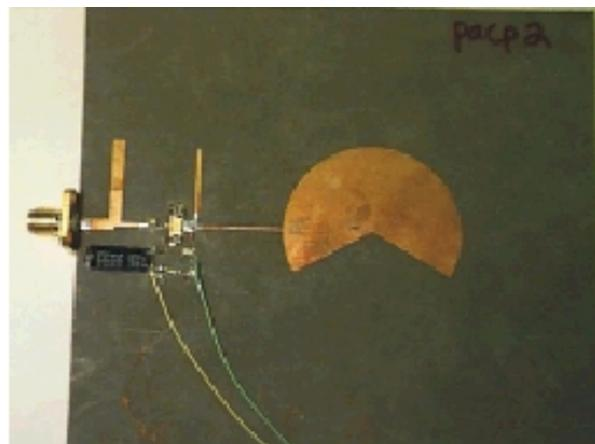
Fig. 1. Class F power amplifier with integrated circular patch antenna.
