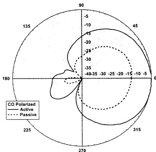
Fig. 8. Measured radiation patterns of active and reference receivers.
