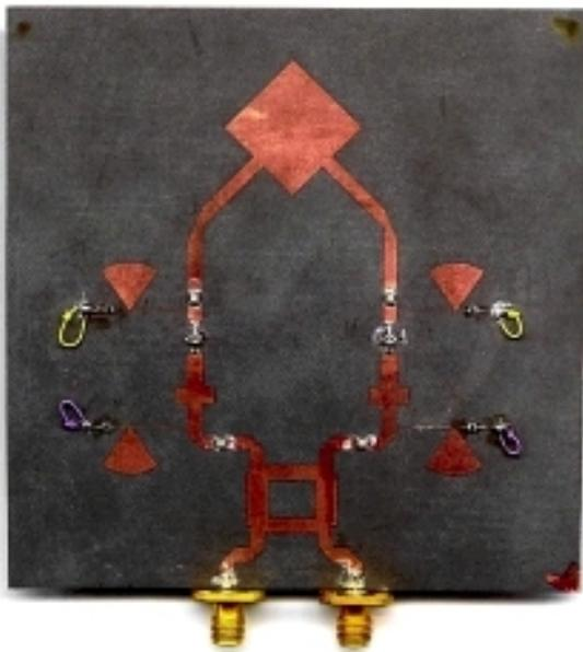
Fig. 5. Photograph of the integrated low noise receiver.
