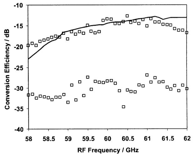
Fig. 10. Measured (marks) and simulated (line) conversion efficiency of the quasi-Yagi antenna SOM.
