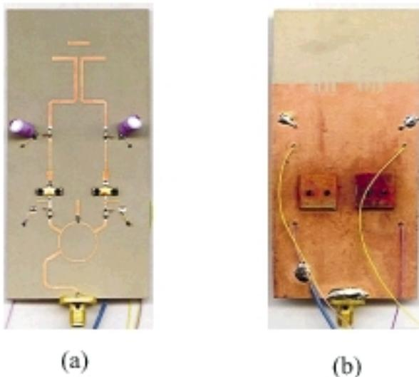
Fig. 3. Push—Pull PA with integrated Quasi-Yagi Antenna.
