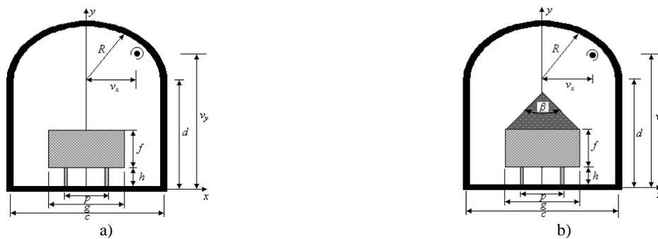
Fig.15 - Mathematical model of mine pit when empty wagon a) and when loaded wagon b) is inside.
