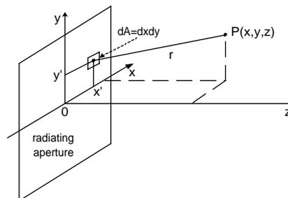
Fig.1. Geometry used in calculation of Gaussian beam radiation
