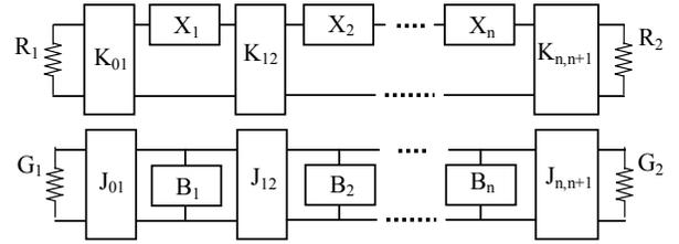
Fig. 4 Filter prototypes using impedance/admittance inverters
