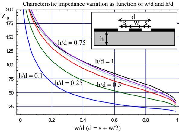
Fig. 3 Dispersion and variation of effective permittivity and characteristic impedance for CPW for  $\epsilon_r = 2.323$ ,  $h = 635 \mu\text{m}$ ,  $s = 200 \mu\text{m}$ ,  $w = 1600 \mu\text{m}$
