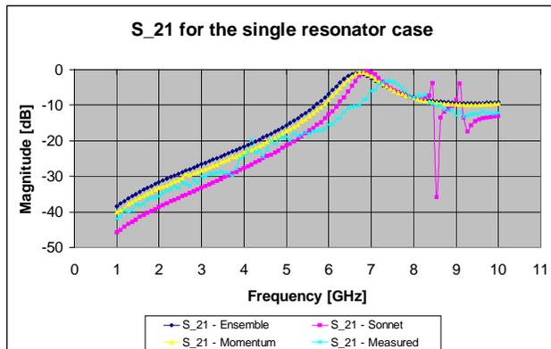
Fig. 6 Comparative data for an single CPW resonator case, using most known microwave CAD software
