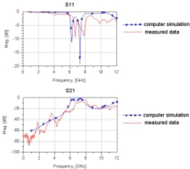
Fig. 5 Comparative design of an single and an double CPW resonator: computer simulation and measured data
