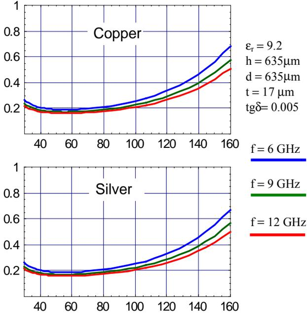
Fig. 2 Dispersion characteristics of attenuation constant as function of characteristic impedance for different metal layer
