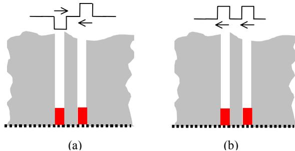
Fig. 1 CPW slot excitation: a) even mode b) odd mode
