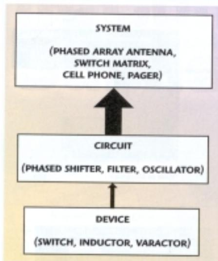
Fig. 1. Typical RF MEMS chain
