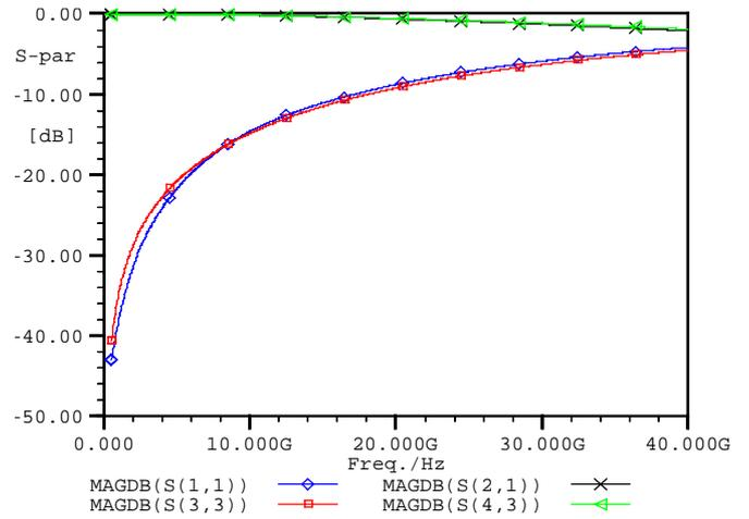
Fig. 6. S-parameters of the EM simulated and lumped element modeled switch in the up-state
