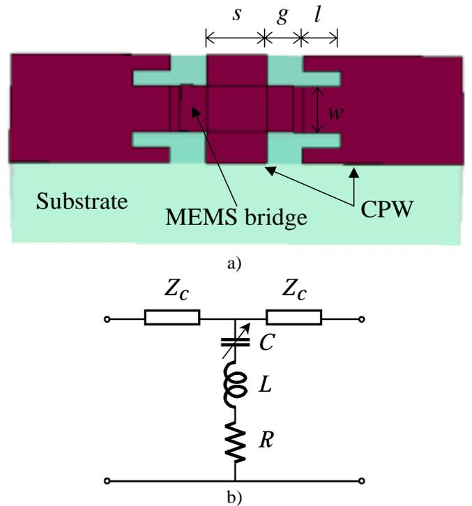
Fig. 5. A typical inductively-tuned MEMS shunt switch a), and an equivalent lumped element model b)
