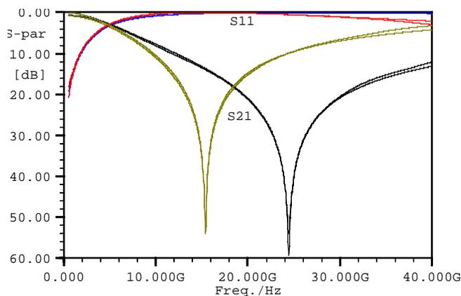
Fig. 7. EM simulated and lumped element modeled S-parameters for the switch in the down-state
