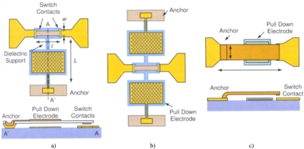
Fig. 3. Broadside series MEMS switch and inline series MEMS switch [9]
