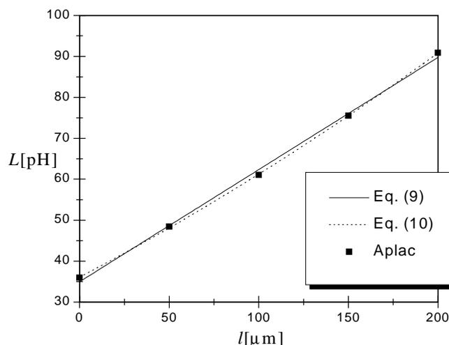
Fig. 8. Inductance of the lumped element model as function of the length of the tuning section
