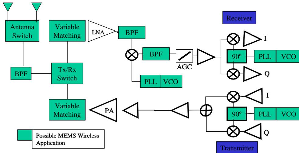
Fig. 2. Schematic of a transceiver with MEMS application
