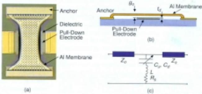
Fig. 4. Raytheon MEMS capacitive shunt switch [9]
