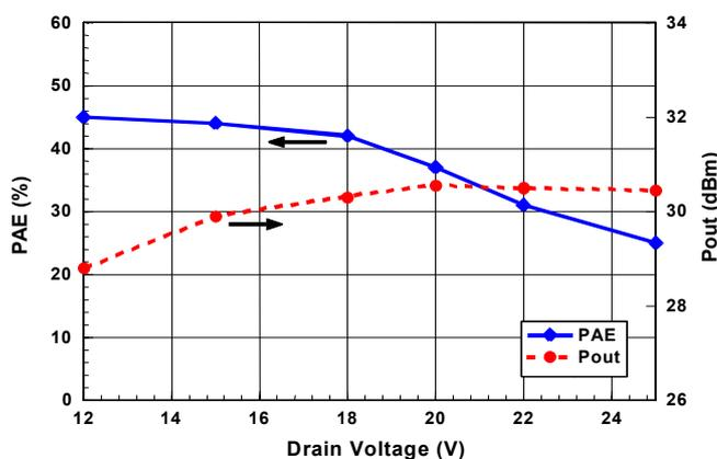
Fig. 7 Measured large-signal performance versus drain bias voltage at 7.25 GHz for the AlGaIn/GaN HFET power amplifier integrated with the microstrip circular sector antenna ( $P_{in}=23$  dBm).
