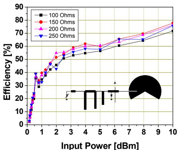
Fig. 14 Overall efficiency of the proposed rectenna with the planar-fed circular sector antenna as a function of the input power at point A.
