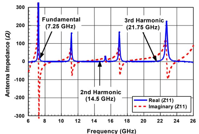
Fig. 3 The resonant characteristic of the microstrip circular sector antenna on RT/Duroid substrate with dielectric constant of 10.2 and thickness of 10 mils ( $Z_{11} = Z_{ANT}$ ).
