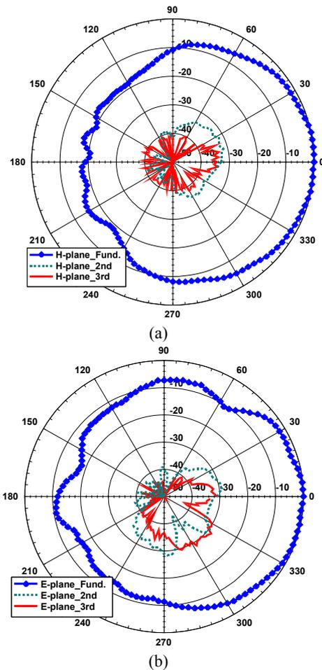
Fig. 8 Measured radiation patterns at the fundamental of 7.25 GHz, second, and third harmonic frequencies for the AlGaIn/GaN HFET power amplifier integrated with the microstrip circular sector antenna. (a) H-plane. (b) E-plane.
