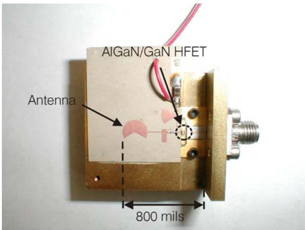
Fig. 4 Photograph of the AlGaIn/GaN HFET power amplifier integrated with the microstrip circular sector antenna on the test jig.
