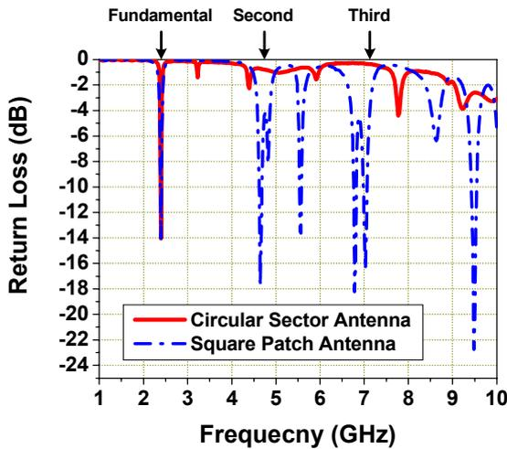
Fig. 10 Measured return losses of the microstrip circular sector and square patch antennas.
