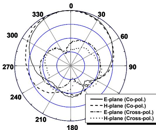
Fig. 12 Radiation patterns of the coaxial-fed circular sector antenna.
