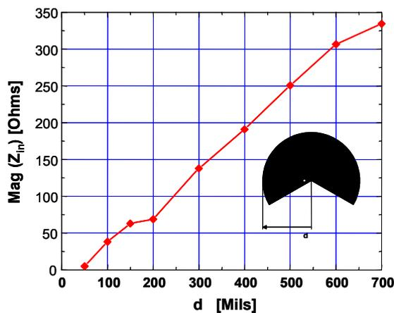
Fig. 11 Antenna input impedance of the coaxial-fed circular sector antenna as a function of the distance from the center of the antenna.
