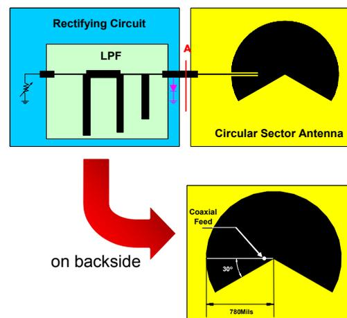
Fig. 13 Rectenna layouts with the coaxial-fed circular sector antenna fed either a planar feedline or a coaxial feedline from back side.
