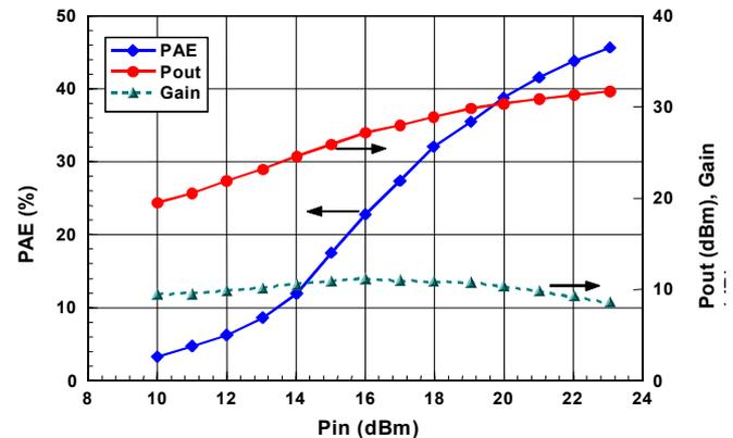
Fig. 2 Measured load-pull large-signal performance for a 1 mm-wide AlGaIn/GaN HFET.
