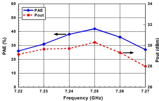
Fig. 6 Measured large-signal performance as a function of frequency for the AlGaIn/GaN HFET power amplifier integrated with the microstrip circular sector antenna ( $V_{DS}=18$  V,  $V_{GS}=-5$  V, and  $P_{in}=23$  dBm).
