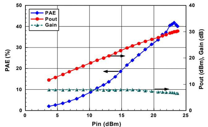
Fig. 5 Measured large-signal performance with respect to input power at 7.25 GHz ( $V_{DS}=18$  V and  $V_{GS}=-5$  V).
