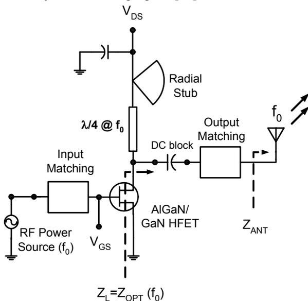
Fig. 1 Schematic of the AlGaIn/GaN HFET power amplifier integrated with microstrip antenna as a RF front-end application. Measured antenna impedance ( $Z_{ANT}$ ) is directly transformed to optimum load impedance ( $Z_{OPT}$ ) for efficiency.
