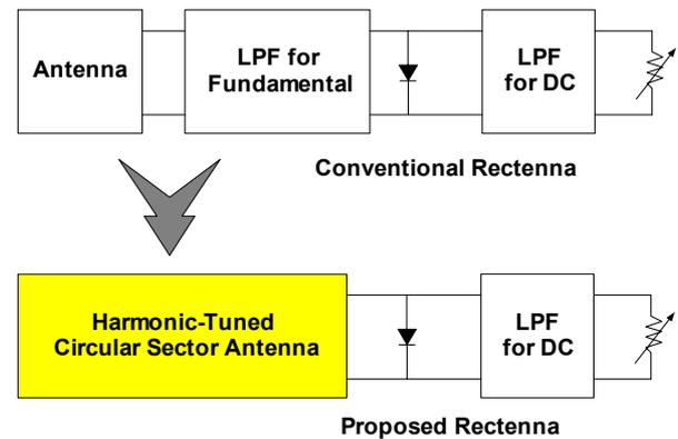
Fig. 9 Block diagram of the conventional and the proposed rectenna system based on the active integrated antenna.
