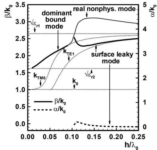
Fig. 15 Dispersion characteristics of a modified conductor-backed slotline ⑤ in Fig. 1, when slot width  $w=6$  mm, substrate thicknesses  $h_1=6$  mm,  $h_2=12$  mm, and permittivities  $\epsilon_{r1}=2.6$ ,  $\epsilon_{r2}=7$  and  $\epsilon_{r3}=1$ .
