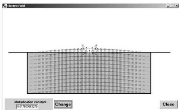
Fig. 22 Electric field of the mode on the slotted waveguide specified in Fig. 21.
