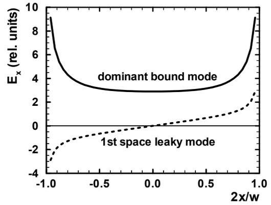
Fig. 7 Transversal electric field component within the slot of the slotline specified in Fig. 6 when  $h/\lambda_0=0.012$ .
