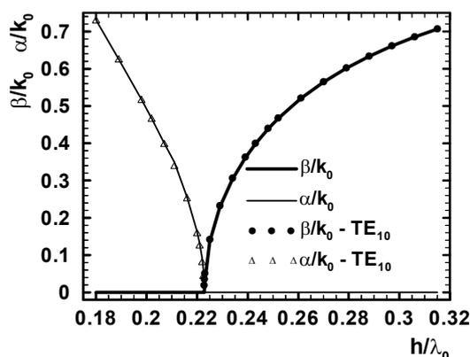
Fig. 21 The dispersion characteristic of the mode on the slotted rectangular waveguide compared with the characteristic of  $TE_{10}$  mode. The slot width is 1 mm, and the internal dimensions are  $22.86 \times 10.12$  mm.
