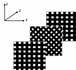
Fig. 1. Carbon Fibre Composite ply organisation (0°/45° “Composite A” or 0°/90° “Composite B”)
