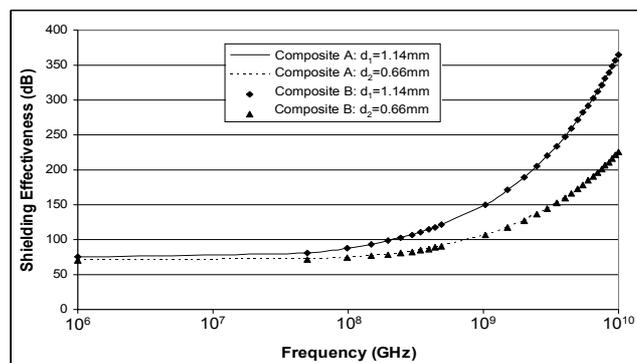
Fig. 4. Composite A and Composite B simulated shielding effectiveness using plane wave theory
