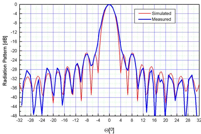
Figure 7. Measured and simulated radiation pattern at 24.1 GHz
