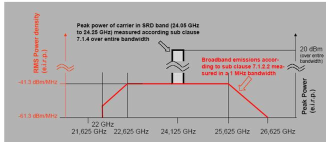
Figure 1. Transmitter maximum radiated peak power density (e.i.r.p) mask for equipment operating in the 22GHz to 26.625GHz
