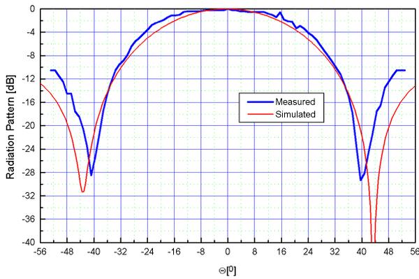
Figure 9. Elevation radiation pattern at frequency of 24.1GHz
