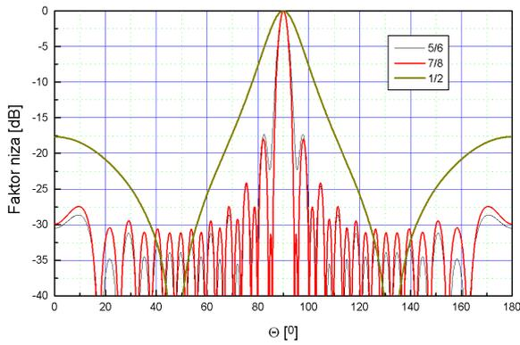
Figure 4. Radiation pattern in H-plane for different values of  $q$
