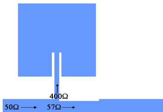
Figure 2. Picture of the  $400\Omega$  patch with the matching network
