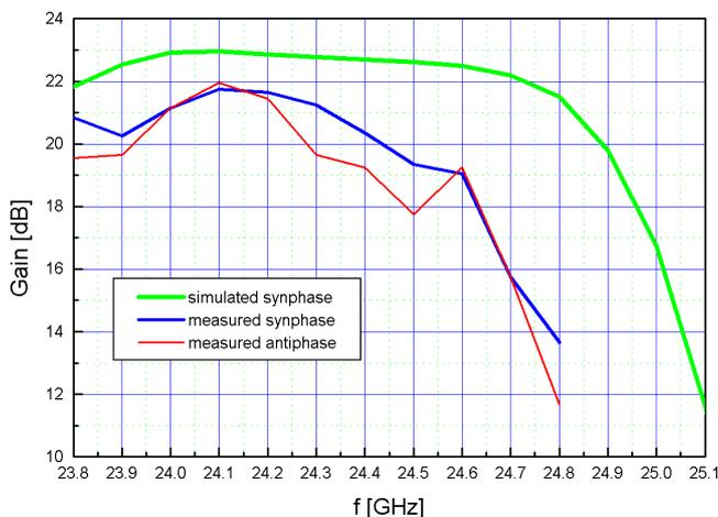
Figure 10. Gain for synphase and antiphase antenna
