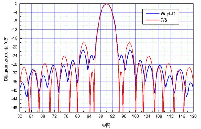
Figure 5. Radiation pattern of array in azimuth (H-plane) obtained by electromagnetic simulation at  $f=24.1\text{GHz}$
