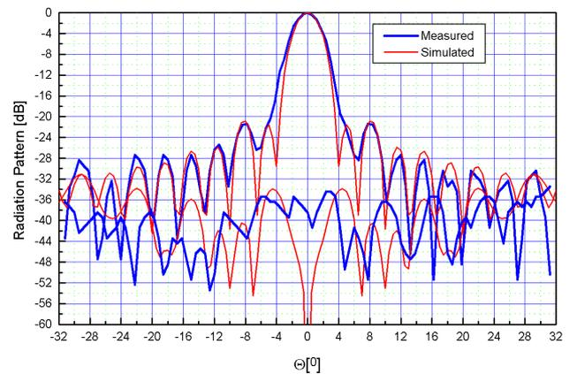
Figure 8. Co-polar and cross-polar radiation pattern at 24.1GHz
