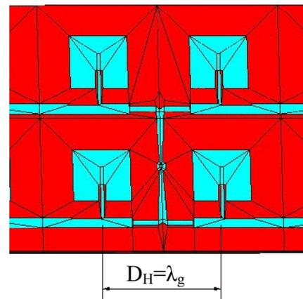
Figure 3. Meshed middle part of synphase antenna array with the feeding network (WIPL-D)
