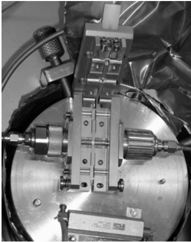
Fig. 1. Photograph of the transistor test fixture (Maury Microwave TTF mod. MT950G) mounted on the thermal chuck
