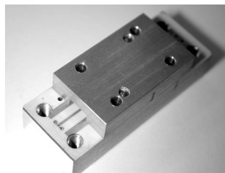
Fig. 3: Photograph of the empty test mount (top) and a lowpass filter on extended substrate in the test mount. Center: opened block with filter, bottom: assembled test setup.
