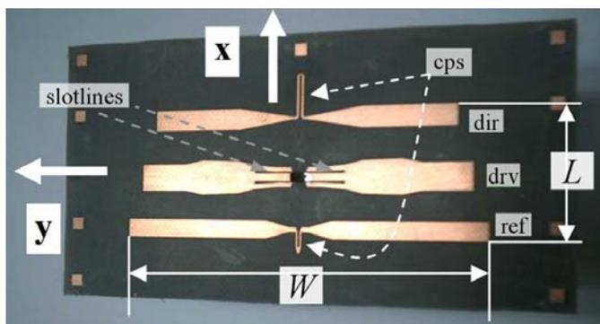
Fig. 3. Realized novel Yagi-Uda antenna with straight tuned dipoles (scalable).
