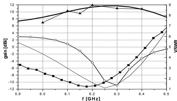
Fig. 5 Gain and SWR of realized Yagi antenna with tuned dipoles
