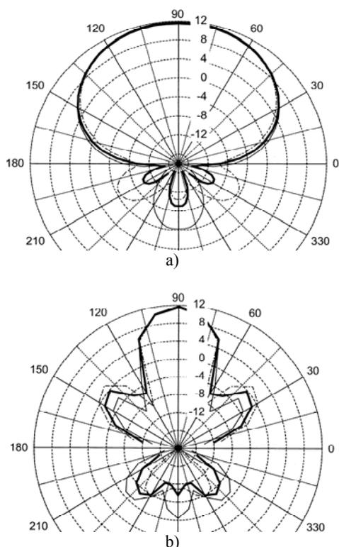
Fig. 4. Radiation pattern [6] of fullwave Yagi antenna with tuned dipoles in:
