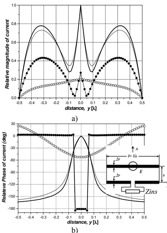
Fig. 2. Current distribution along fed and passive wire dipole in air
