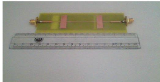
Fig.5. Prototype model of offset slot EBG LPF
