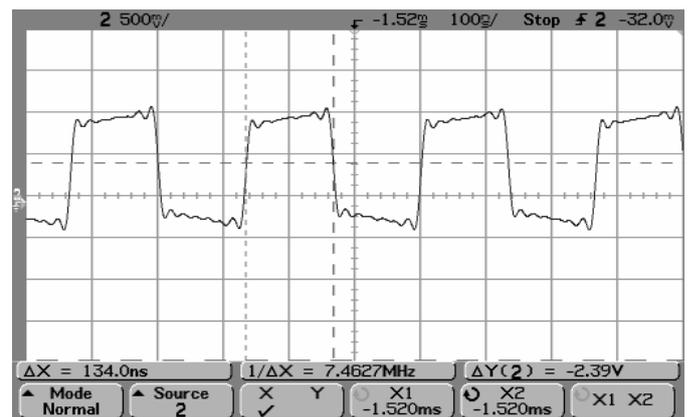
Fig. 10. Output of the first channel of the receiver kit for the 1024 – carriers – DPSK system as shown by the oscilloscope.
