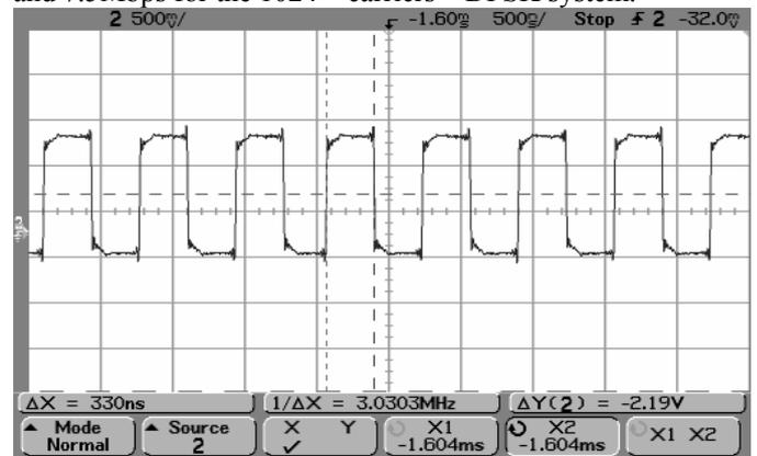
Fig. 8. The output of the first channel of the 16 – carriers – BPSK receiver kit as depicted by the oscilloscope.
