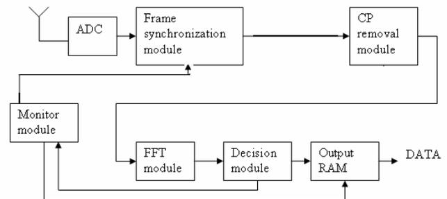
Fig. 3. Block diagram of the architecture of the receiver circuits.
