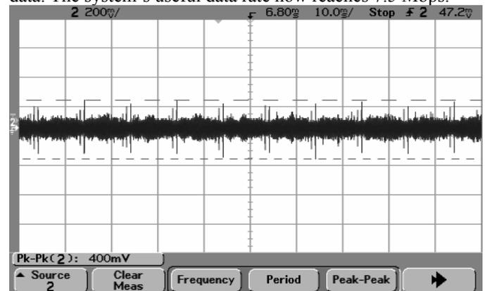
Fig. 4. Screenshot of powerline noise as taken by an oscilloscope.
