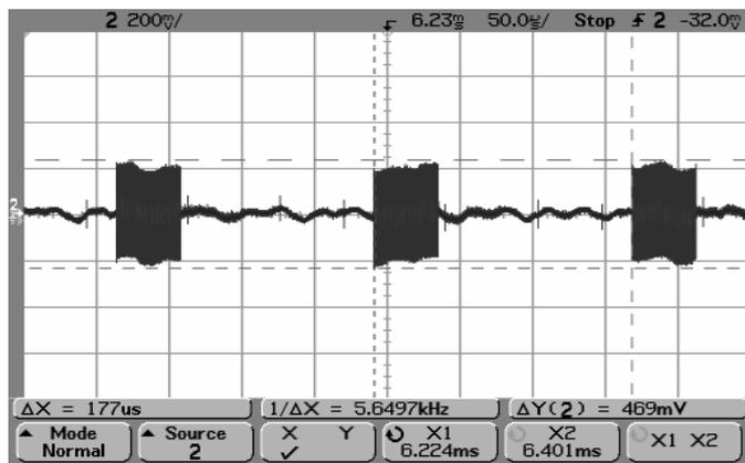
Fig. 7. Signal at the input of the receiver for the 1024 – carriers – BPSK system. SNR is measured at 1.4dB.
