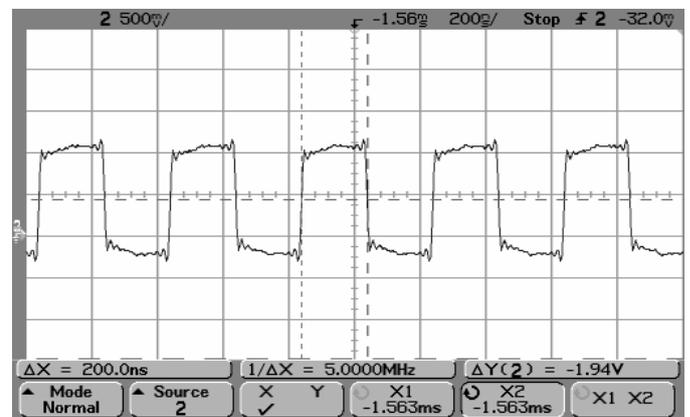
Fig. 9. Retrieved data sequence at the output of the receiver development kit for the 1024 – carriers – BPSK system.
