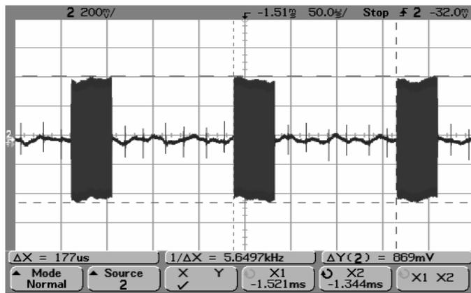
Fig. 6. Signal at the input of the receiver for the 1024 – carriers – DPSK system. SNR is measured at 6.5dB.
