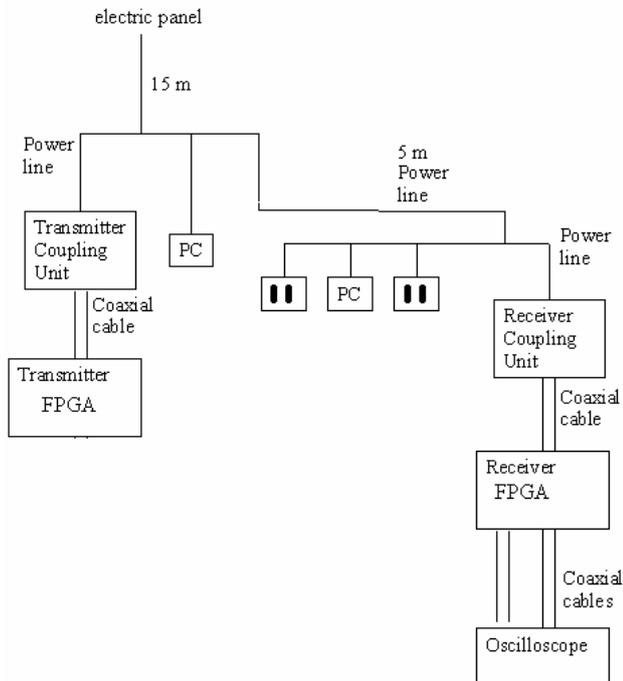
Fig. 1. Setup to evaluate the OFDM systems and powerline network topology.
