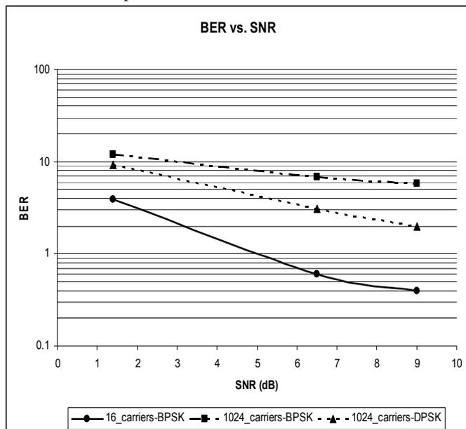
Fig. 11. Analytical BER performance of the three OFDM systems under varying SNR.
