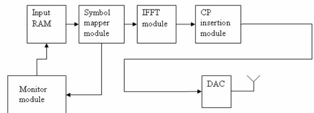
Fig. 2. Block diagram of the architecture of the transmitter circuits.
