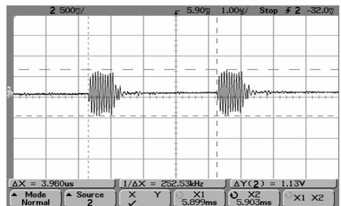
Fig. 5. Signal at the input of the receiver for the 16 – carriers – BPSK system. SNR is measured at 9dB.
