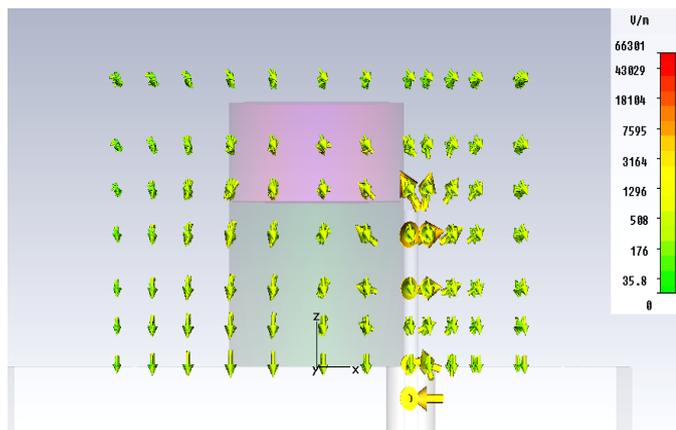
Fig. 5 Electric field distribution in dual segment CDRA
