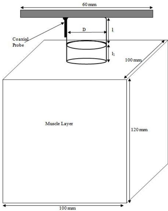
Fig. 7 Dual segment CDRA in direct contact with muscle layer
