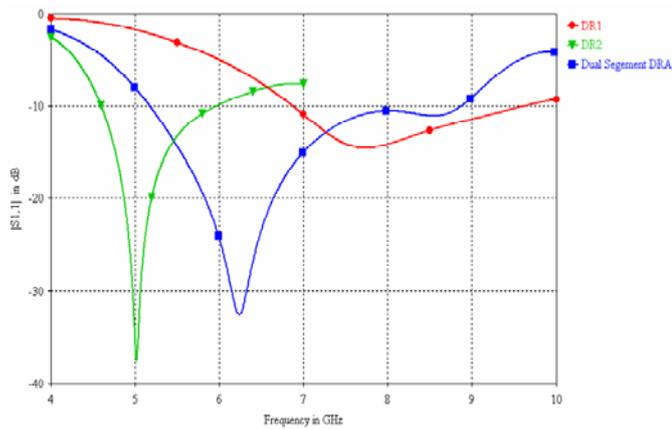
Fig. 2 Return loss versus frequency performance of dual segment CDRA
