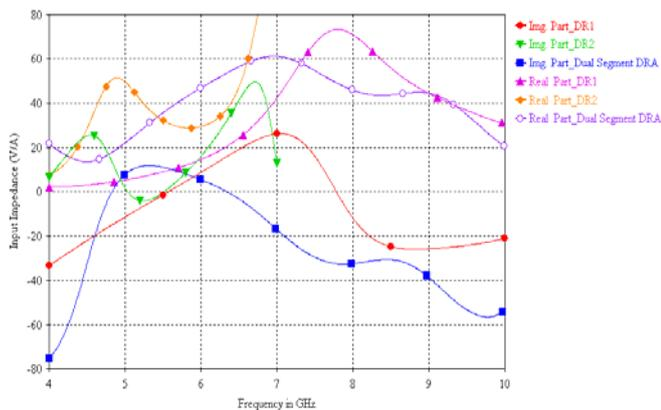
Fig. 3 Input impedance versus frequency curves of dual segment CDRA
