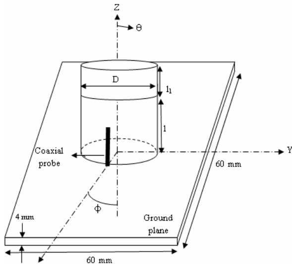
Fig. 1 Geometry of dual segment CDRA
