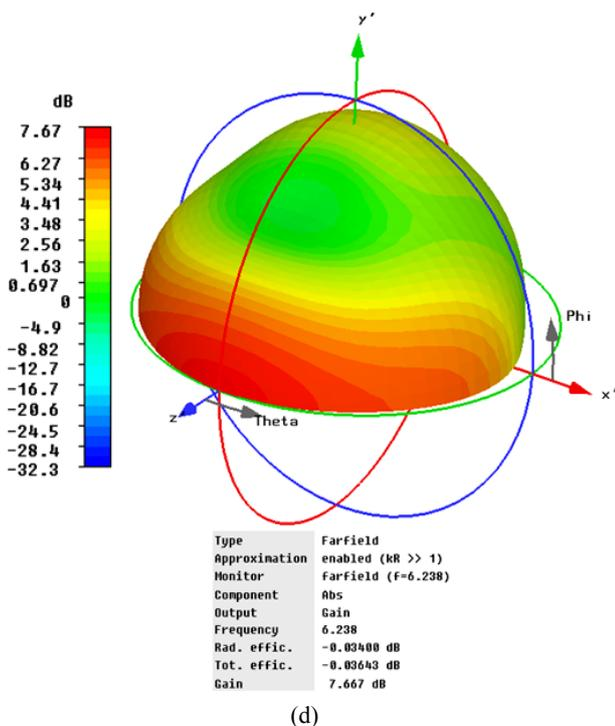
Fig. 6 Far field patterns of dual segment CDRA (a) in X-Z plane (b) in Y-Z plane (c) in X-Y plane (d) 3-D pattern
