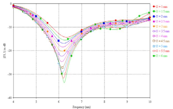
Fig. 4 Effect of variation in length of upper dielectric segment on the return loss versus frequency characteristics of dual segment CDRA
