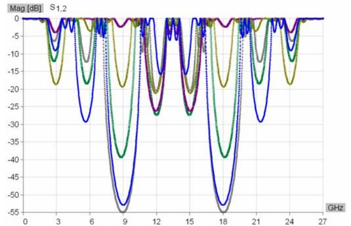
Fig. 2.  $S_{12}$  of cascade of four identical cells made of nine sections obtained for five random choices of section impedances.
