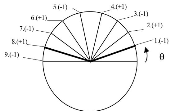
Fig. 3. Position of band-gaps depends on angle (bold lines mark desirable bandgaps) (-) or (+) correspond to boundaries of the dispersive polynomial
