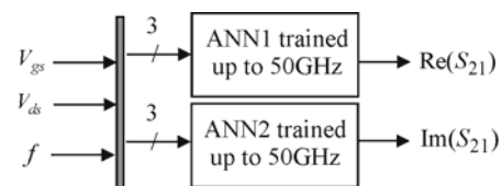
Fig. 4. Basic small-signal bias-dependent neural model for FinFET forward transmission coefficient.
