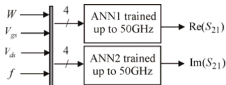
Fig. 1. Small-signal bias-dependent neural model for the forward transmission coefficient of HEMTs with different gate width.
