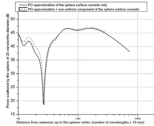
Fig. 7. Power scattered by the conductive sphere 20 wavelengths diameter along the distance from the sphere vertex up to the point observation on the axis coming through the sphere center
