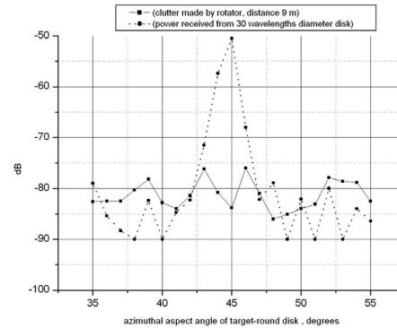
Fig. 8. Experimental detection of circular disc of 30 wavelengths diameter at 9 m distance by the TRX MS against aspect angle
