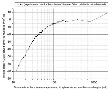
Fig. 6. Data shown in Fig.4 multiplied by 4-th degree of distance from the horns up to the sphere vertex
