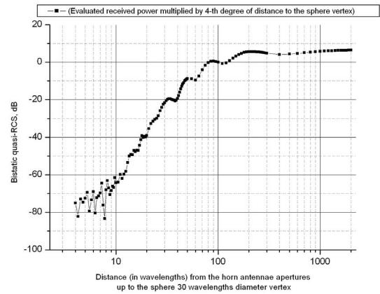
Fig.3. Evaluated (shown in Fig.2) received power in the near-field radar model multiplied by 4-th degree of distance from the radar antennae apertures up to the sphere vertex
