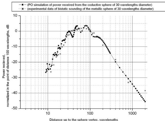
Fig. 2. PO modeling and experimental results for sounding the sphere of 30 wavelengths diameter
