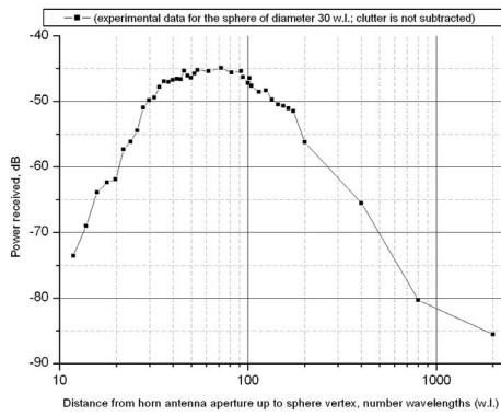
Fig. 5. Experimental results for sounding the same (as Fig. 3) sphere for 12 – 2000 wavelengths distance
