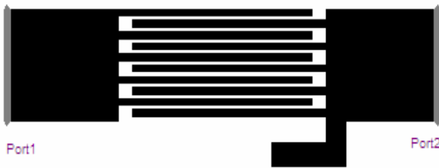
Fig.3. One-dimensional CRLH Unit cell unit cell with input and output
