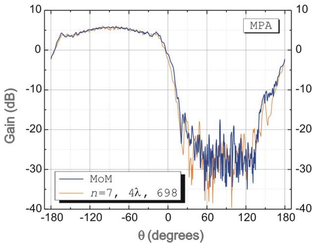
Fig. 9. Gain, Mom vs PDM solution of  $4\lambda$  model, iteration 7
