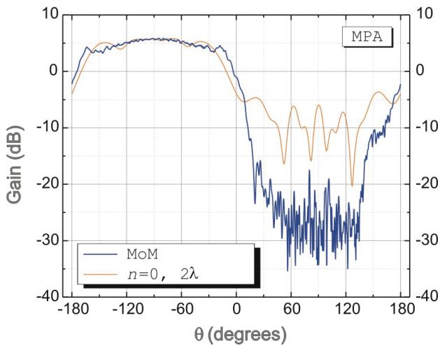
Fig. 10. Gain, Mom vs PDM solution of  $2\lambda$  model, iteration 0
