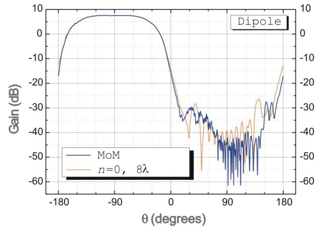
Fig. 17. Gain, Mom vs PDM solution of  $8\lambda$  model, iteration 0
