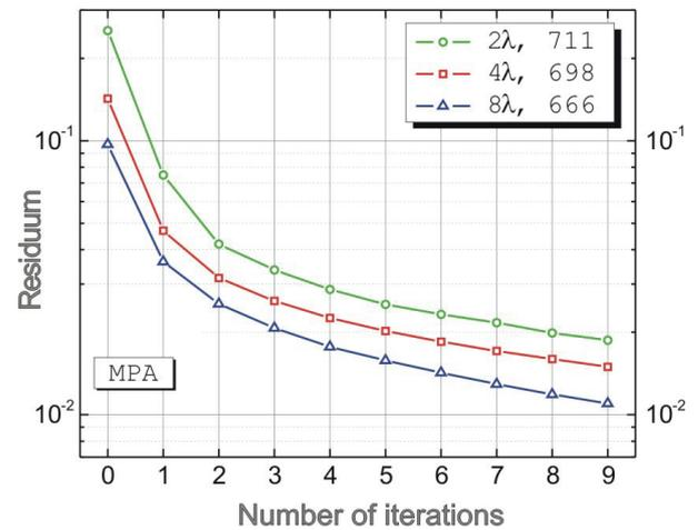
Fig. 3. Residuum as a function of size of MoM area
