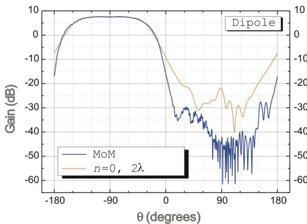
Fig. 15. Gain, Mom vs PDM solution of  $2\lambda$  model, iteration 0
