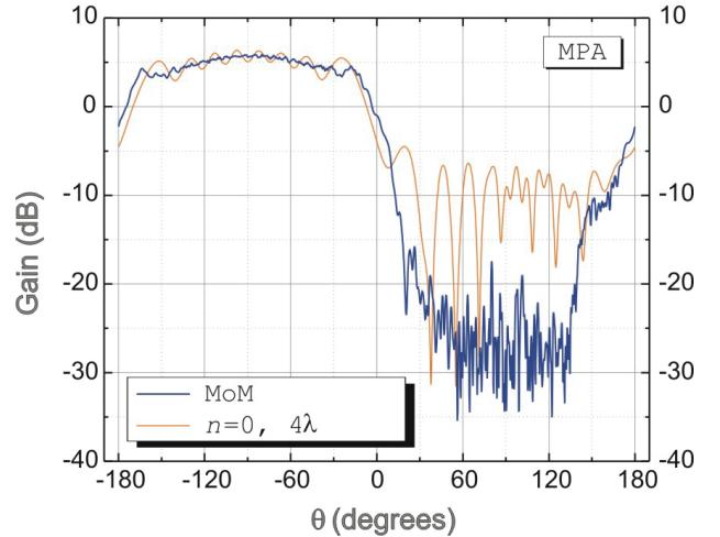
Fig. 6. Gain, Mom vs PDM solution of  $4\lambda$  model, iteration 0
