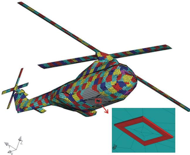
Fig. 1. Model of MPA on the helicopter, with 12022 patches, 95730 BFs,  $4\lambda$  MoM area, and 698 groups of patches in PO area
