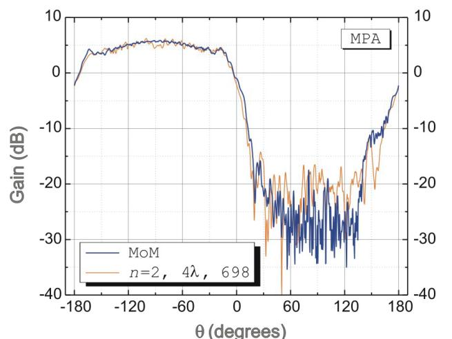
Fig. 8. Gain, Mom vs PDM solution of  $4\lambda$  model, iteration 2
