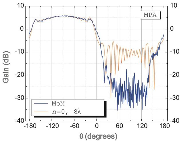
Fig. 11. Gain, Mom vs PDM solution of  $8\lambda$  model, iteration 0
