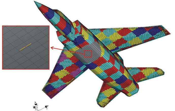
Fig. 12. Model of the dipole on the airplane, with 13072 patches, 104279 BFs,  $4\lambda$  MoM area, and 316 groups of patches in PO area
