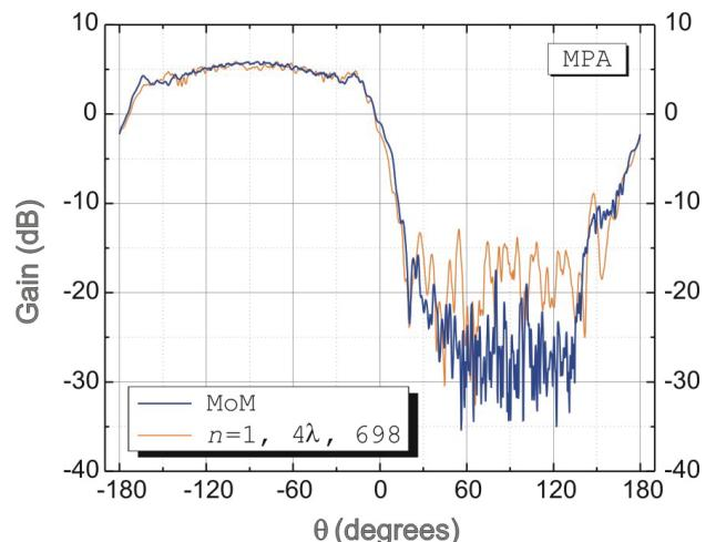
Fig. 7. Gain, Mom vs PDM solution of  $4\lambda$  model, iteration 1
