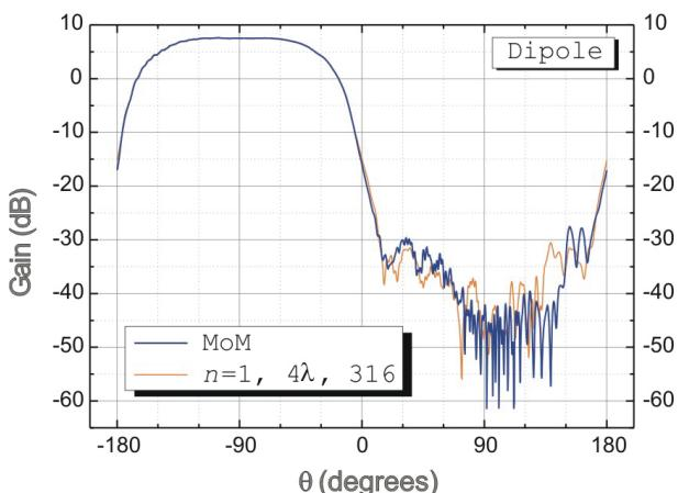
Fig. 19. Gain, Mom vs PDM solution of  $8\lambda$  model, iteration 1
