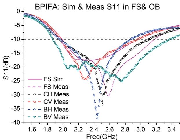
Fig. 9. Measured and simulated  $S_{11}$  for BPIFA in free space and on body locations [45]
