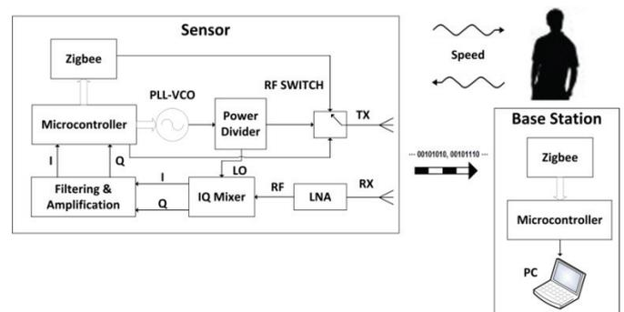
Fig. 1. Simplified block diagram of the contactless health monitoring system
