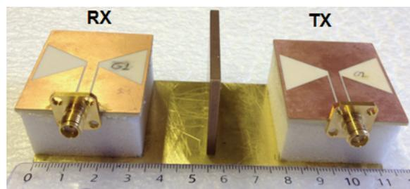
Fig. 3. Prototype of bow-tie TX/RX antenna array for broadband indoor radar applications
