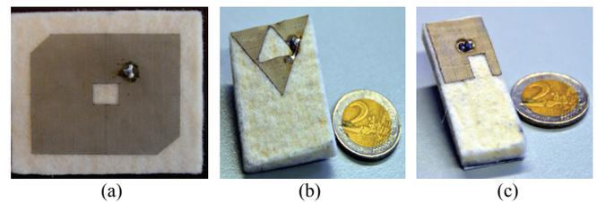
Fig. 4. Fabricated prototypes of the all-textile antennas: (a) narrowband antenna [33], (b) broadband PIFA [38], and (c) dual band PIFA [39]
