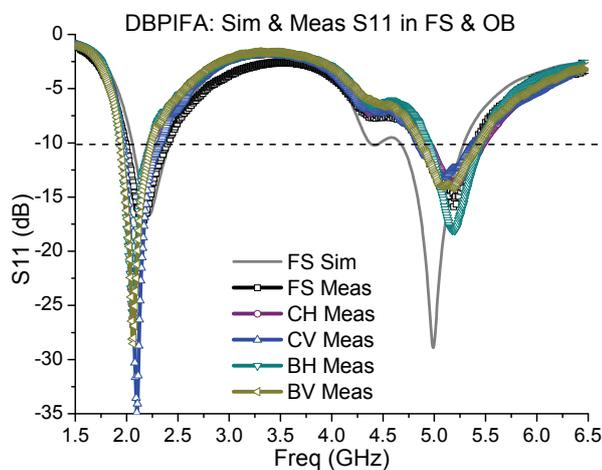
Fig. 10. Measured and simulated  $S_{11}$  for DBPIFA in free space and on body locations [38]
