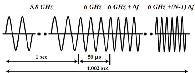
Fig. 2. Designed radar waveform
