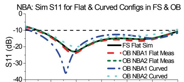
Fig. 8. Measured and simulated  $S_{11}$  and axial ratios for NBA in free space and on phantom [26]
