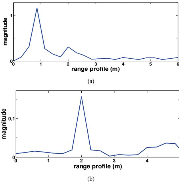
Fig. 5. Range profile of a target at 2 m away the antennas before (a) and after (b) compensation and the calibration
