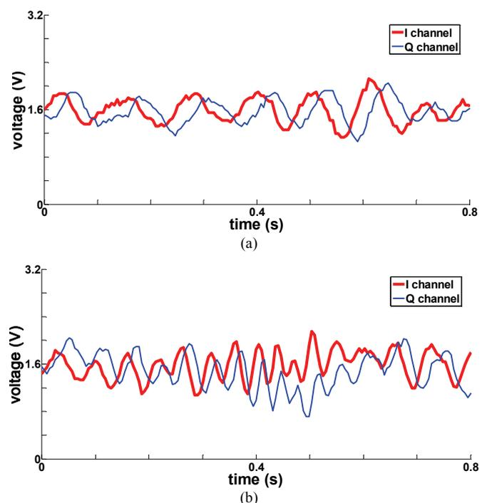
Fig. 6. Speed signal during (a) a walking movement and during (b) a fall event. The frequency of the signal is proportional to the radial velocity of the person during the movement. An inflating mattress has been used when invoking falls. For that reason, the fall speed signals do not stop suddenly but there is also the effect of the rebounds on the mattress
