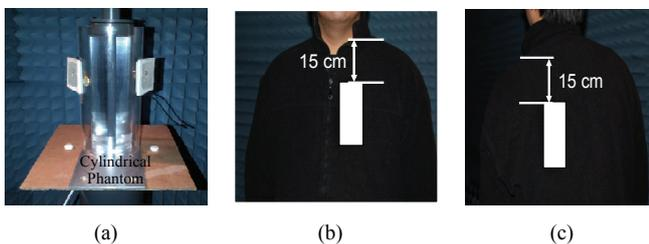
Fig. 7. On-body evaluation setups: (a) on-body phantom, and (b) on a real human volunteer (chest), and (c) back
