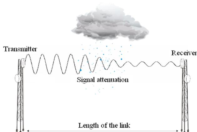
Fig. 1. Signal attenuation of the microwave link, which occurs due to the precipitation occurrence
