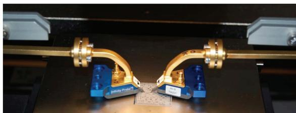
Fig. 16. Circuit under measurement using pico-probes
