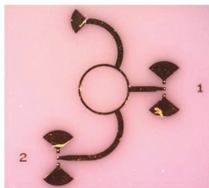
Fig. 18. Microphotograph of the novel ring power divider: S12 measurement configuration
