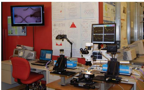
Fig. 15. S-parameter measurement set-up
