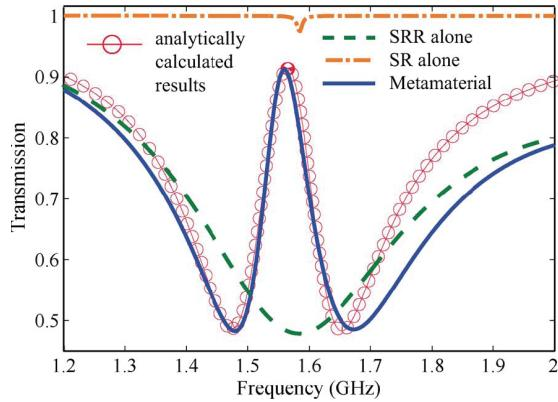
Fig. 11. Simulated transmission through metamaterial consisting only from SRRs, spirals, and both of them combined [6]
