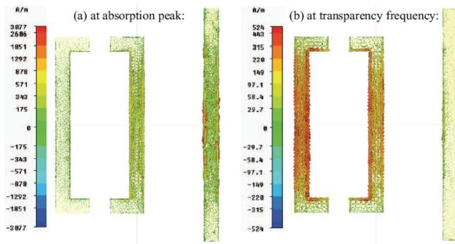
Fig. 6. Current distributions for metamaterial shown in Fig. 5a at (a) absorption peak; (b) transparency frequency [3]
