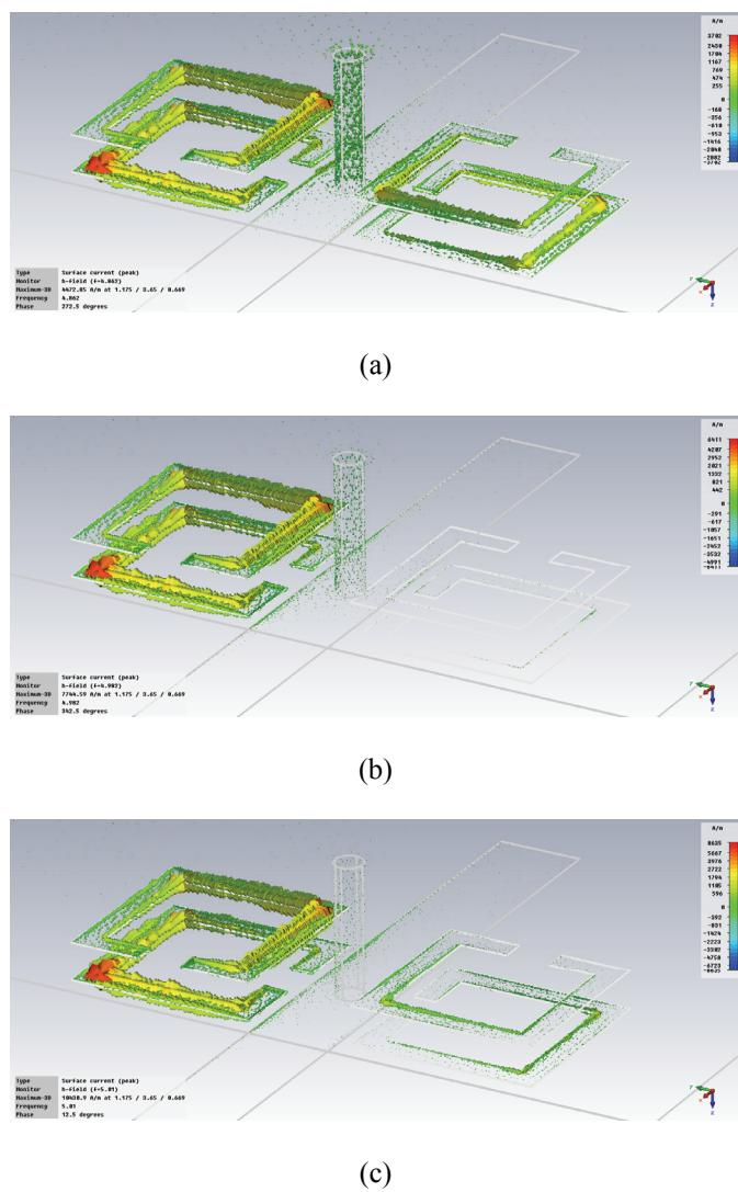
Fig. 16. Current distribution at EIT-like response at characteristic frequencies denoted in Fig. 13
