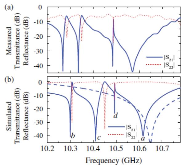
Fig. 7. (a) Measured and (b) simulated transmission and reflection spectrum for the hybrid metal/superconductor EIT metamaterial [5] (a)
