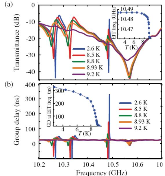
Fig. 9. Control of the group delay by temperature for hybrid metal/superconductor EIT metamaterial [5]
