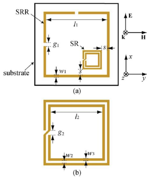
Fig. 10. Polarization independent EIT metamaterial unit cell [6]
