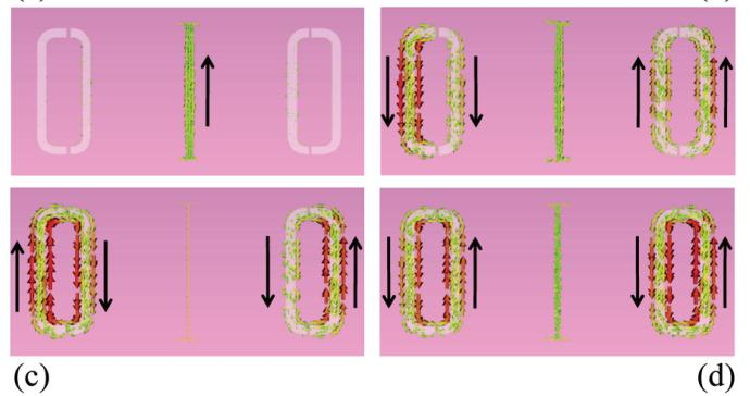
Fig. 8. Current distribution at the characteristic frequencies from Fig. 7a for hybrid metal/superconductor EIT metamaterial [5]
