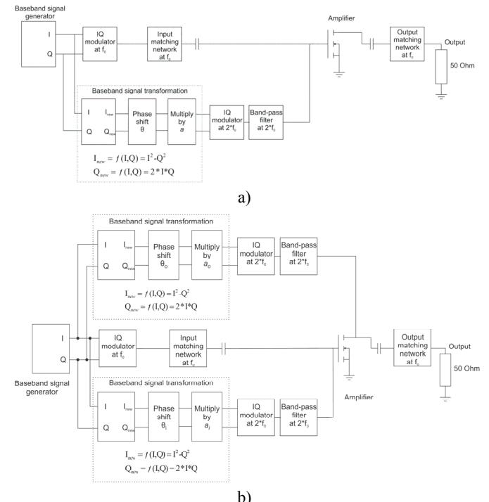
Fig. 1. Schematic diagram of the amplifier linearization with the injection of the second harmonic modulated by the modified baseband signal a) at the input of the amplifier; b) at the input and output of the amplifier
