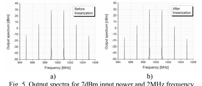
Fig. 5. Output spectra for 7dBm input power and 2MHz frequency spacing between spectral components of the QAM signal a) before and b) after linearization
