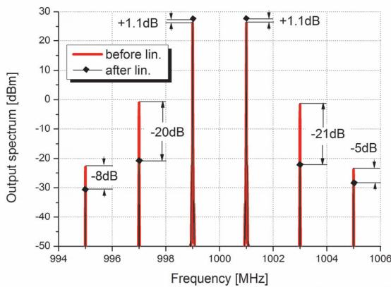
Fig. 9. Output spectra before and after linearization for 3dBm input power and 2MHz frequency spacing between spectral components of the QAM signal
