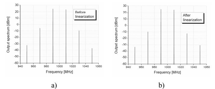
Fig. 4. Output spectra for 0dBm input power and 20MHz frequency spacing between spectral components of the QAM signal a) before and b) after linearization
