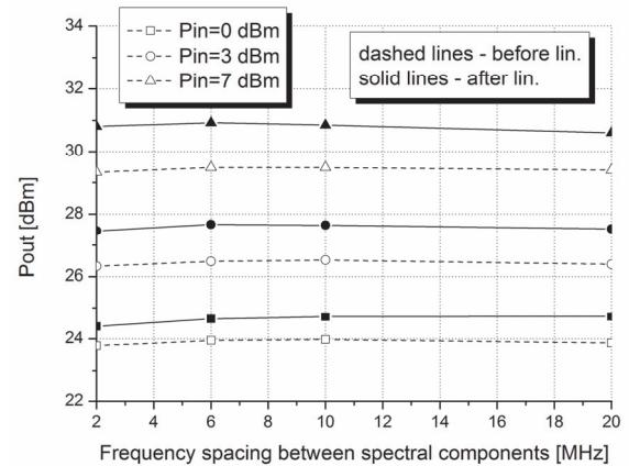
Fig. 10. Output power of fundamental signals before and after the linearization
