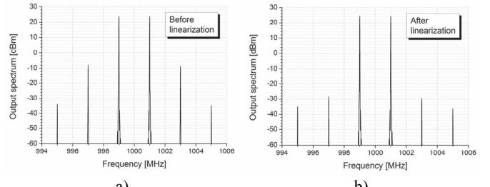
Fig. 3. Output spectra for 0dBm input power and 2MHz frequency spacing between spectral components of the QAM signal a) before and b) after linearization
