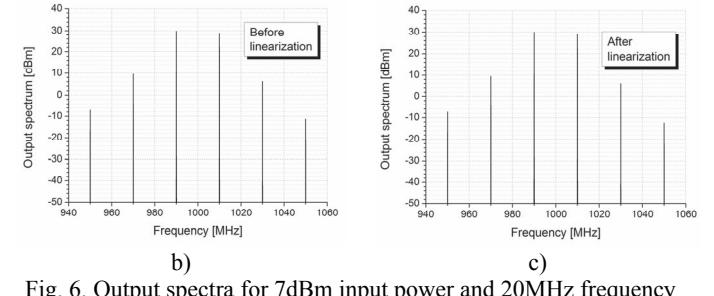
Fig. 6. Output spectra for 7dBm input power and 20MHz frequency spacing between spectral components of the QAM signal a) before and b) after linearization
