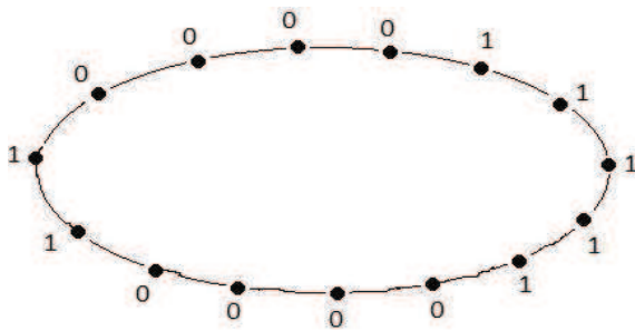
Fig. 8. PSO optimized thinned elliptic array (46.66% filling)
