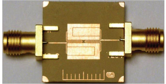
Fig. 7. Photo of the realized microstrip EABPF<sub>Δ</sub>
