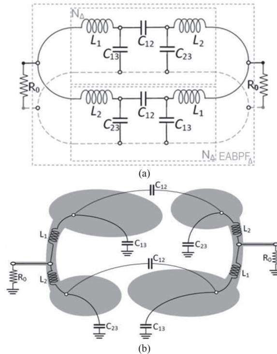
Fig. 6. (a) Circuit diagram of EABPF<sub>Δ</sub> and (b) the corresponding general planar topology (for better visibility, the reference ground plane and the dielectric layer are not shown)
