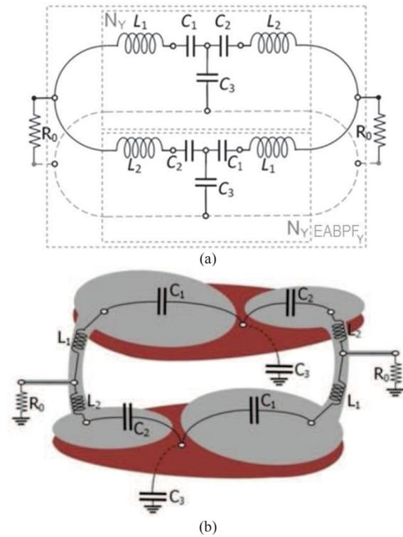
Fig. 5. (a) Circuit diagram of EABPF<sub>Y</sub> and (b) the corresponding general planar topology (for better visibility, the reference ground plane and the dielectric layers are not shown)
