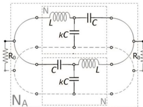
Fig. 1. Circuit diagram of a BABPF formed by an antiparallel connection of two identical asymmetrical subnetworks  $N$
