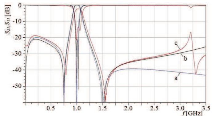
Fig. 8. Filter's S-parameters comparison between: a) scaled EABPF<sub>Δ</sub> prototype; b) ideal TL model; c) measured results
