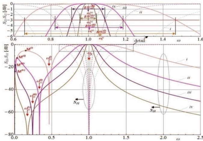
Fig. 2. Frequency characteristic of  $S_{21}$  and  $S_{11}$  parameters of four BABPF prototypes from Table 1
