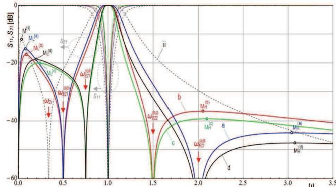
Fig. 4. Comparison of S parameter frequency characteristics of four EABPFs from Table 3 and a basic BABPF (ii) from Table 1
