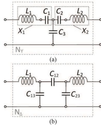
Fig. 3. Two mutually equivalent extended subnetworks: a) with capacitors in Y configuration; b) with capacitors in  $\Delta$  configuration
