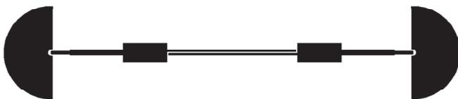
Fig. 7. Wideband microstrip DC block filter layout
