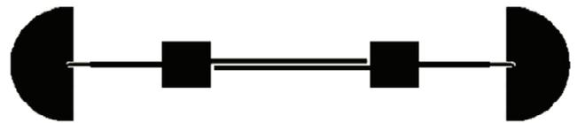
Fig. 9. Narrowband microstrip DC block filter layout
