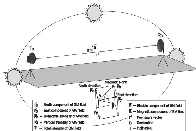
Fig. 1. Radio-relay link and components of geomagnetic field
