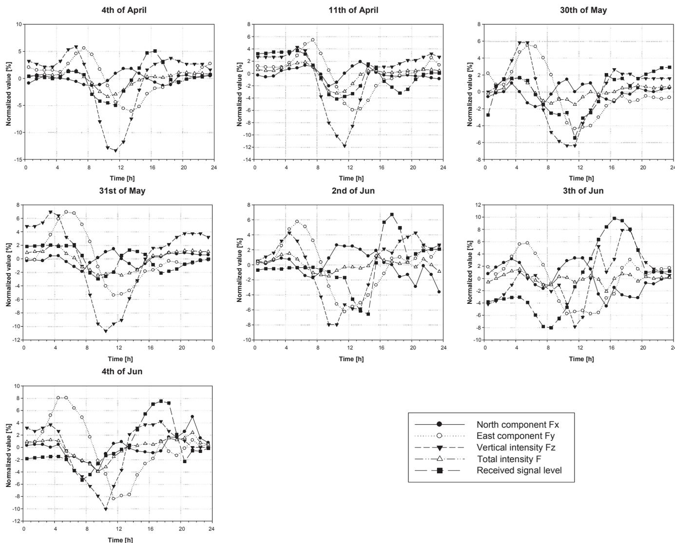
Fig. 3. Hourly variations of received signal level and geomagnetic field components
