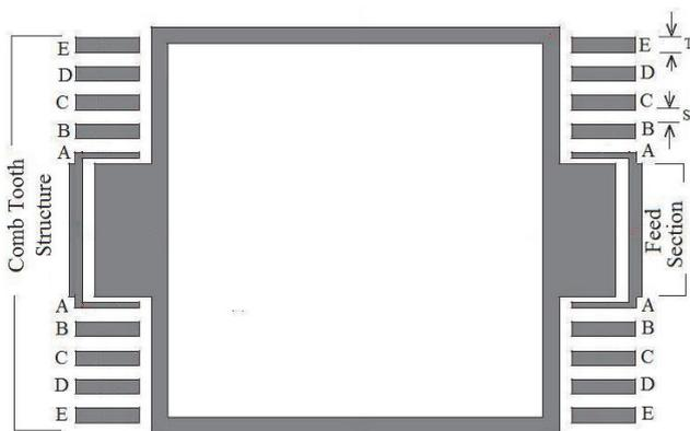
Fig. 4. Layout of the proposed bandpass filter
