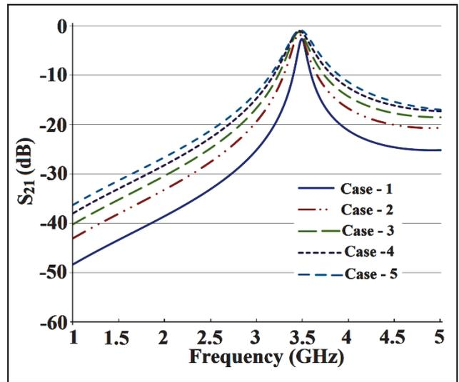
Fig. 5. Insertion loss vs. frequency plot for the layout of proposed filter shown in Fig. 4
