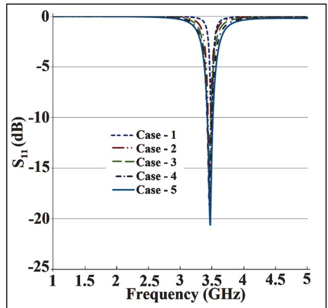
Fig. 6. Reflection loss vs. frequency plot for the layout of proposed filter shown in Fig. 4
