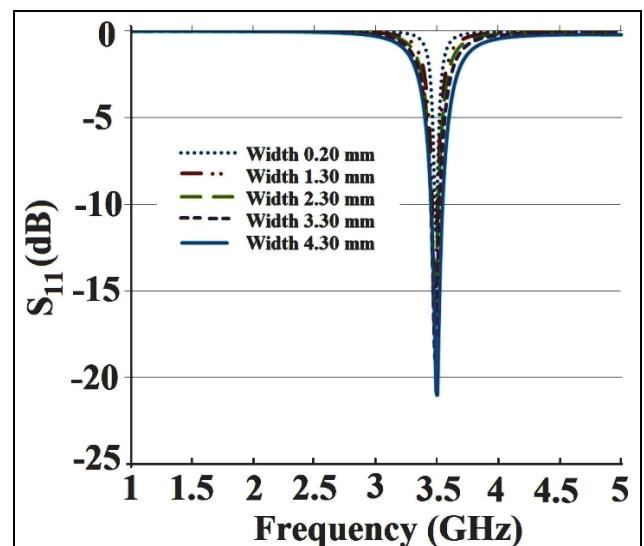
Fig. 3. Reflection Loss vs. frequency plot for the layout of Fig. 1
