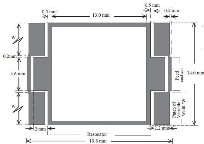
Fig. 1. Layout of the bandpass filter with variable width coupling patch
