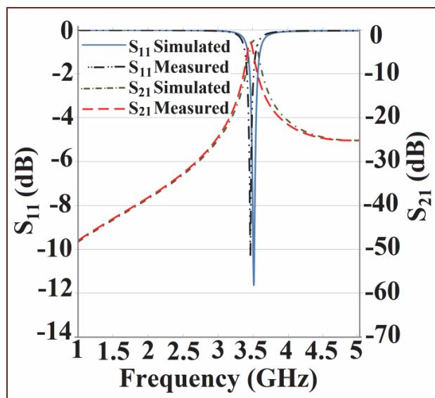
Fig. 8. Simulated and measured result for case -1
