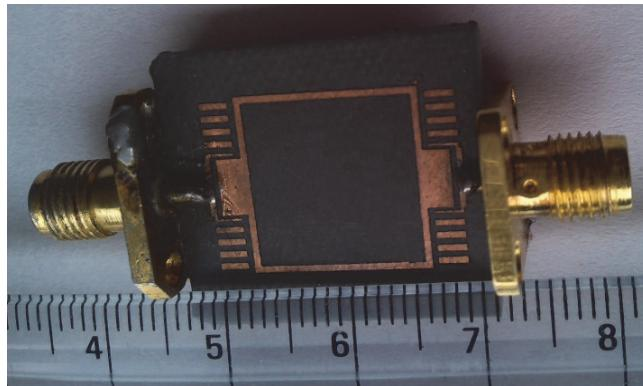
Fig. 7. Fabricated prototype of proposed Bandpass filter
