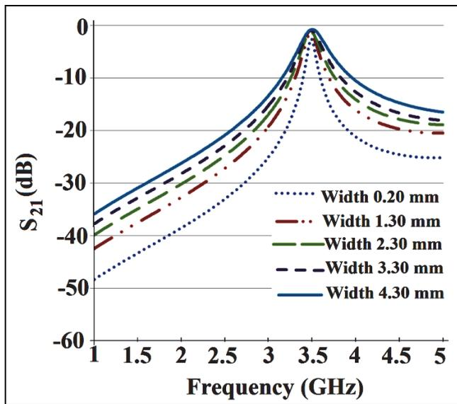
Fig. 2. Insertion loss vs. frequency plot for the layout of Fig. 1
