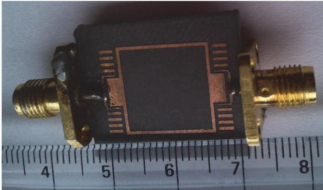
Fig. 7. Fabricated prototype of proposed Bandpass filter
