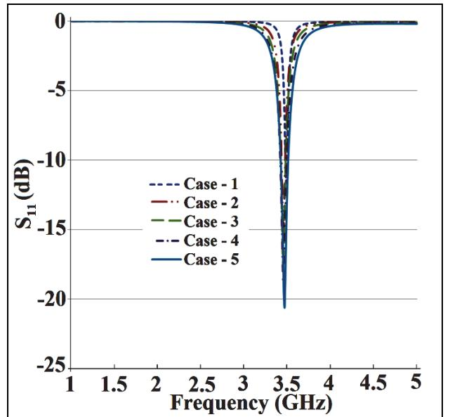
Fig. 6 .Reflection loss vs. frequency plot for the layout of proposed filter shown in Fig. 4
