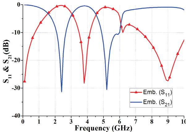
Fig. 9. Simulation result of embedded radial dual bandstop filter
