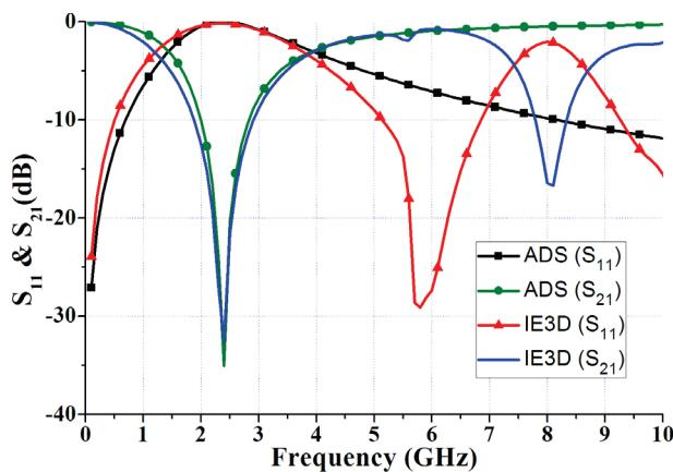
Fig. 2. Simulated results of lumped circuit and microstrip radial structure  $f_r = 2.4$  GHz
