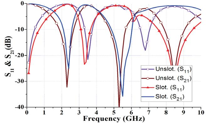
Fig. 7. Simulated results of unslotted and slotted dual bandstop filter
