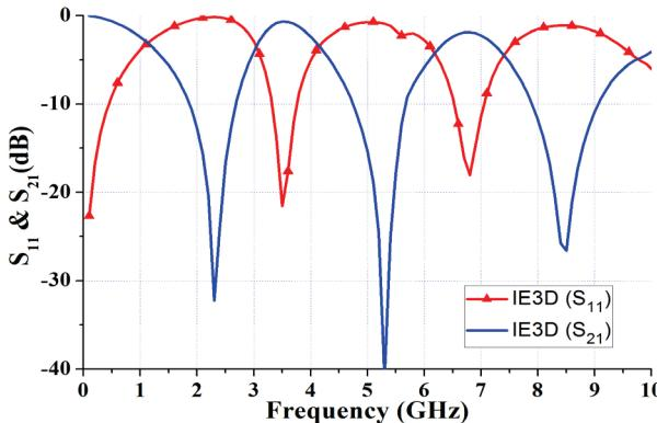
Fig. 5. Simulated result of microstrip dual bandstop filter
