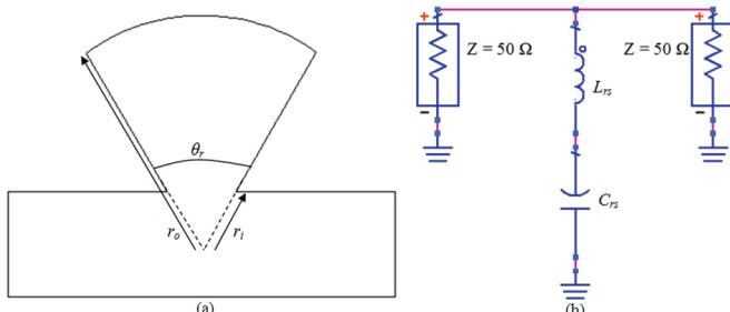
Fig. 1. Bandstop filter and its equivalent circuit model.
