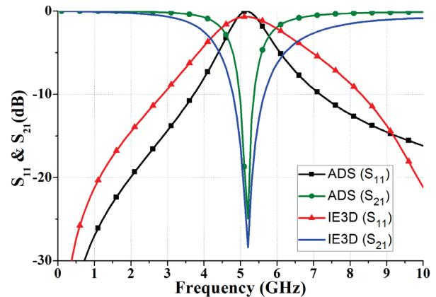
Fig. 3. Simulated results of lumped circuit and microstrip radial structure for  $f_r = 5.2$  GHz
