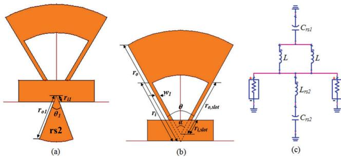
Fig. 6. Slotted radial structure and its equivalent circuit
