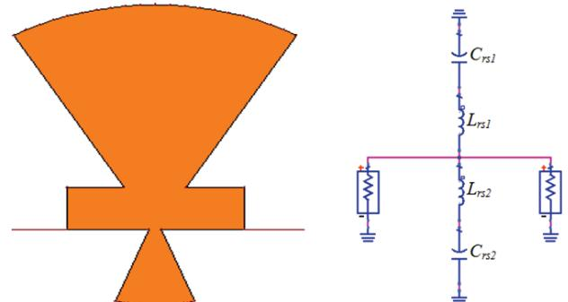
Fig. 4. Dual bandstop filter and its equivalent circuit model
