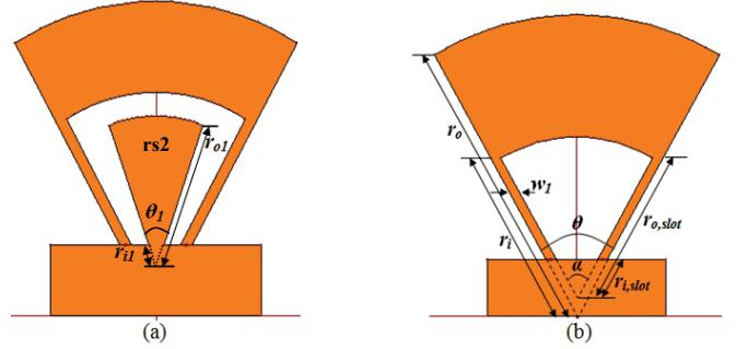
Fig. 8. (a) Embedded radial dual bandstop filter, (b) Slotted section of (a),  $r_{o1} = 6.5$  mm,  $r_{i1} = 1$  mm,  $\theta_1 = 40^\circ$ ,  $r_o = 13.4$  mm,  $r_i = 9.5$  mm,  $\theta = 60^\circ$ ,  $r_{o,slot} = 8.5$  mm,  $r_{i,slot} = 2.3$  mm,  $\alpha = 60^\circ$  and  $w_l = 0.58$  mm
