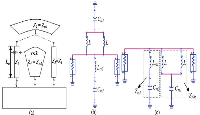
Fig. 10. (a) Proposed model of DBSF, (b) Its equivalent circuit, (c) Simplification of equivalent circuit
