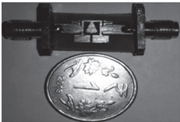
Fig. 8. Fabricated prototype of proposed microstrip LPF
