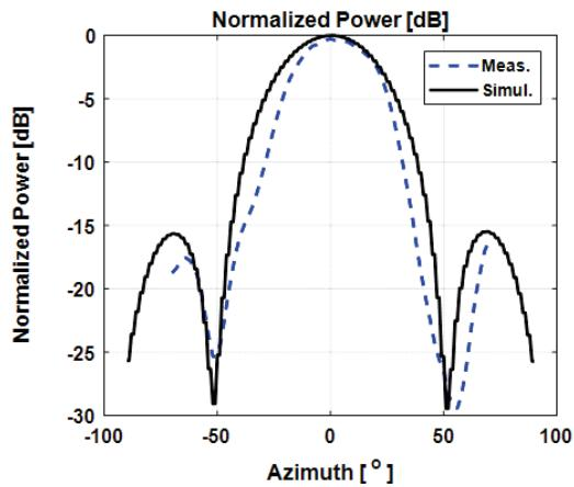
Fig. 8. Simulated and measured RP results in H-plane (azimuth) for linear polarization
