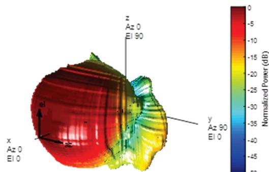
Fig. 13. Measured 3D linear polarized RP
