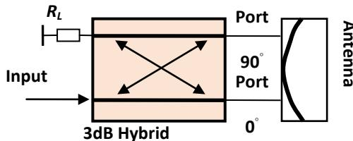
Fig. 3. The antenna feed network using 3dB BLC for circular polarization
