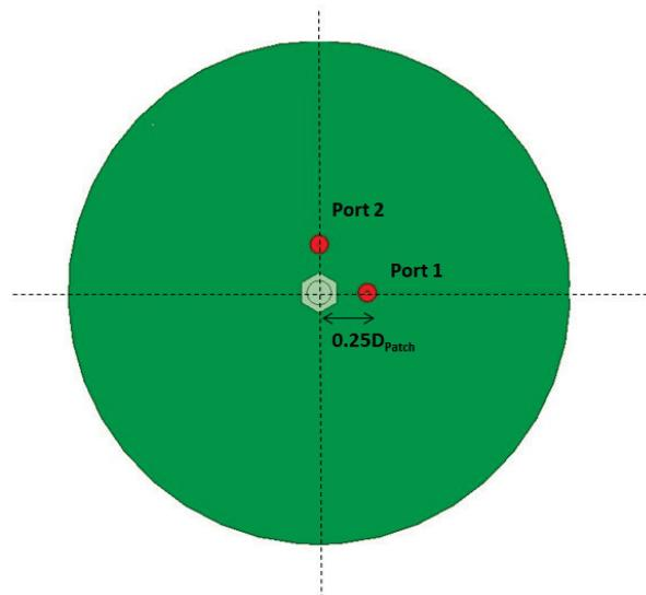
Fig. 2. The location of the feed points of the hybrid antenna for CP
