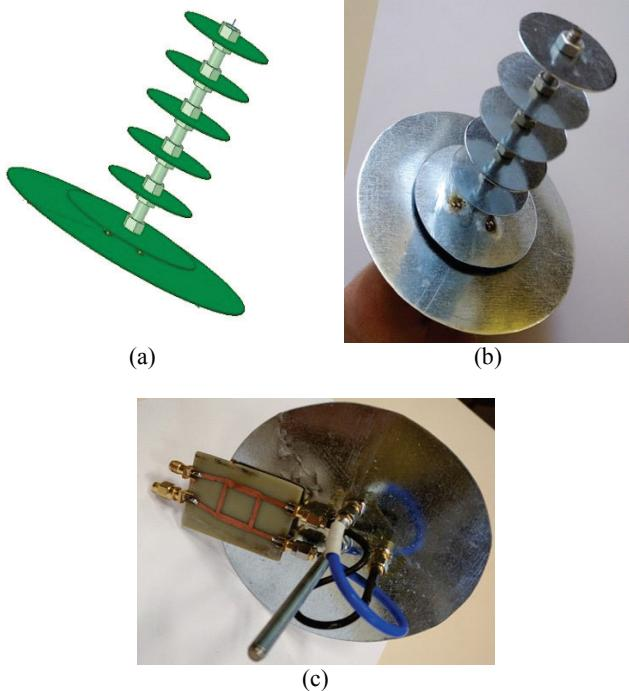
Fig. 4. (a) Simulation model of hybrid antenna, (b) Fabricated model of hybrid antenna, and (c) Feed network realization
