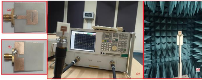
Fig. 3. Proposed sensing antenna prototype for experimental verification: (a): upper patch, (b) lower patch, (c) & (d) setup model
