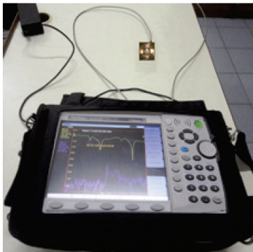
Fig. 8. Experimental set up to measure return loss characteristics of the proposed antenna array
